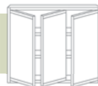
Granville mirror doors open as shown. Door swing cannot be changed.
